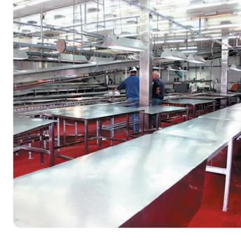
We recommend Ecolabs process 125c for this procedure. It is important to ensure floors are thoroughly rinsed. Floors showing white deposits have been left to drain without chemicals being thoroughly rinsed.
